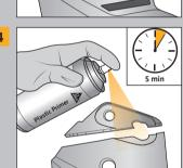
Spray a thin coat of Plastic Primer on both sides, flash-off for 5 min<sup>1)</sup>
