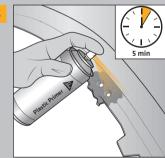
■ Spray a thin coat of Plastic Primer on both sides, flash-off for 5 min¹)
