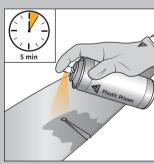
■ Spray a thin coat of Plastic Primer on both sides, flash-off for 5 min<sup>1)</sup>
